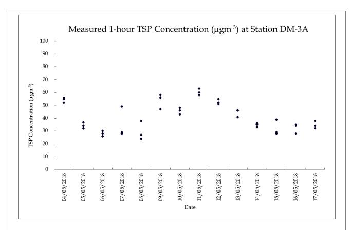
Figure 3: Measured 1-hour TSP Concentration at Station DM-3A between 4 and 17 May 2018
