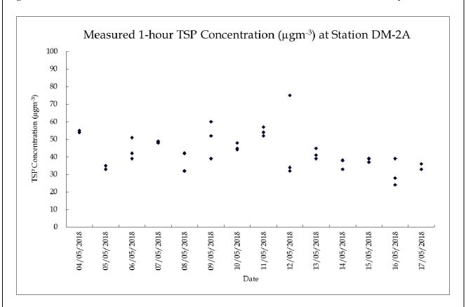
Figure 2: Measured 1-hour TSP Concentration at Station DM-2A between 4 and 17 May 2018
