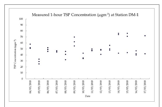
Figure 1: Measured 1-hour TSP Concentration at Station DM-1 between 4 and 17 May 2018
